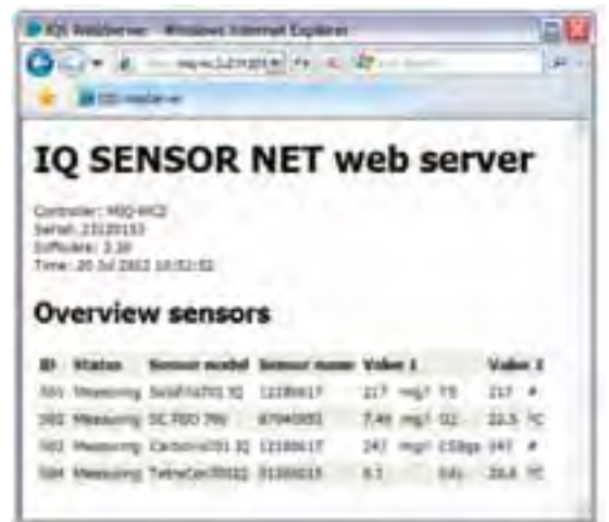
Using a web browser, measured values of the IQ SENSOR NET web server are displayed
